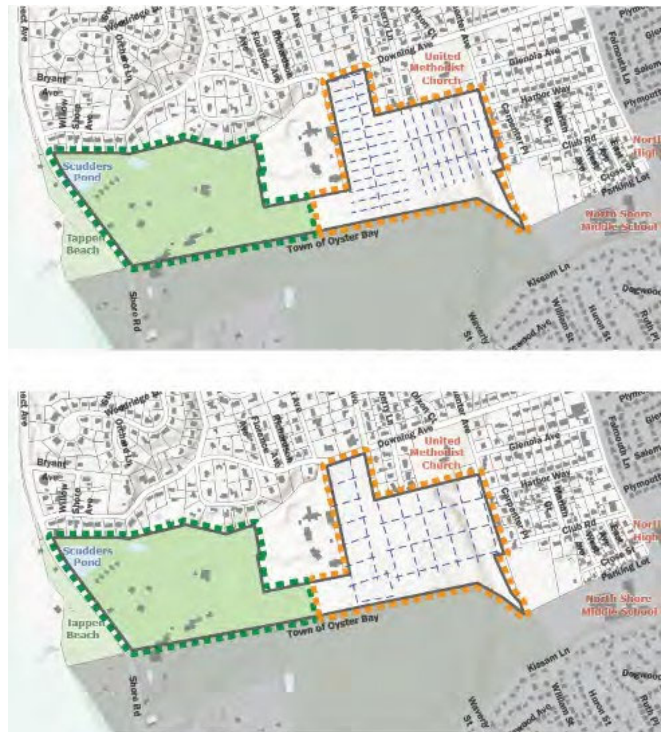
Figure 5-5: Conceptual illustration of a conservation subdivision of the North Shore Country Club. In both scenarios, 50% of the area is preserved open space. The top illustration shows roughly half-acre lots, while the bottom illustration shows roughly 1 acre lots. There are currently no plans to redevelop the country club.
