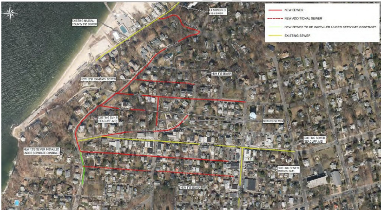
Figure 6-3: Sanitary Sewer Project: Recently Added Sewer Lines
