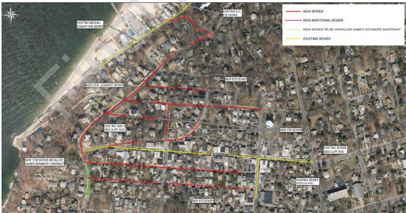
Figure 6-3: Sanitary Sewer Project: Recently Added Sewer Lines
