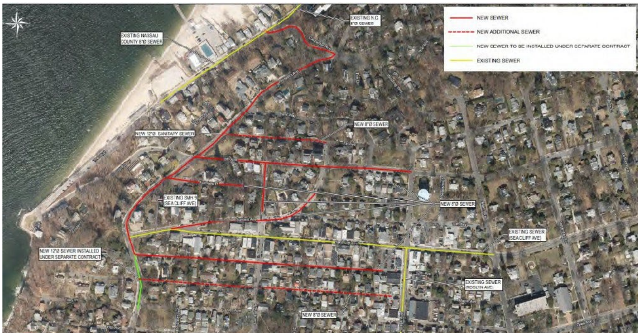
Figure 6-3: Sanitary Sewer Project: Recently Added Sewer Lines
